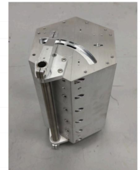
Array with fully assembled tuning system
