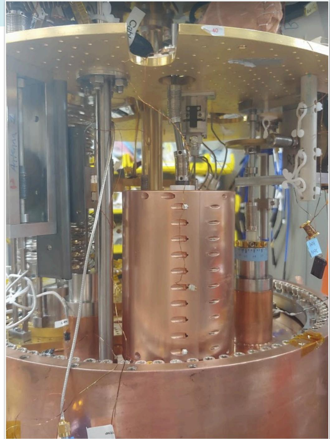
Sidecar sitting on top of the main cavity for Run 1C
