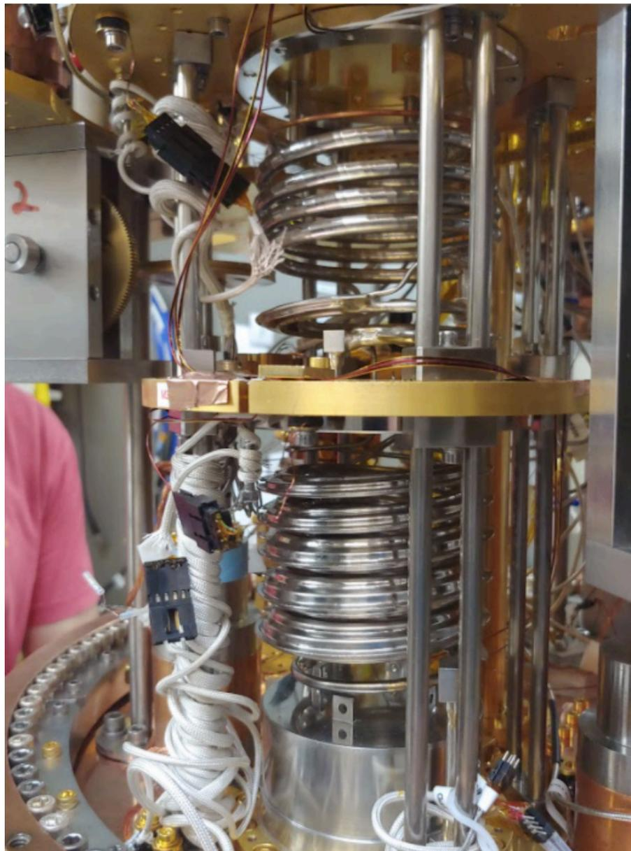
Dilution Refrigerator Mounted to Cavity
